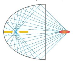
The gap across which the electricity jumps is on the left, inside the reflector. The resultant pressure wave is projected to the right.
